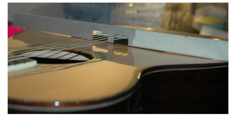
Note the gap under the straight edge showing the collapsed soundboard.
